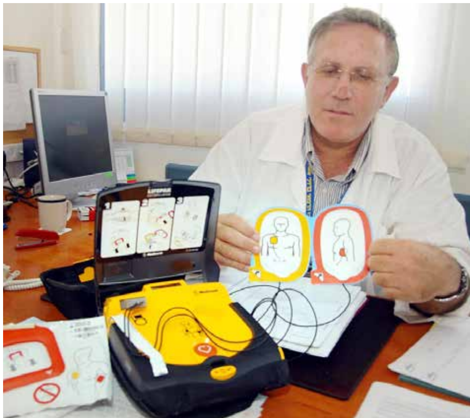
Example of an AED with its components
